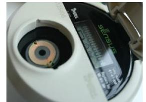
Electronic Register LCD Display
